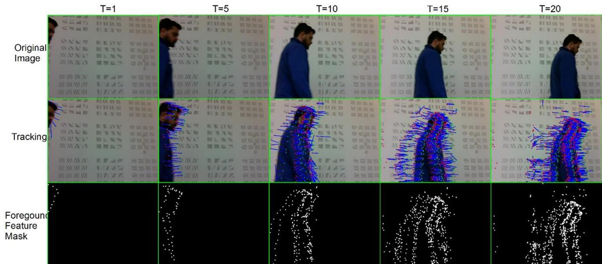
Figure 5.7: Results from the proposed method of tracking motion input from the background subtraction module previously and without clustering feature points. (Top row) original images, (middle row) tracking using Lucas-Kanade pyramid optical flow algorithm and (bottom row) foreground feature mask generated without clustering
