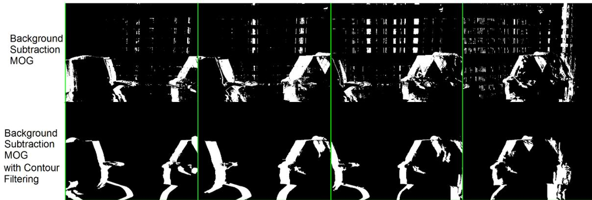
Figure 4.3: Results of Background Subtraction using Mixture of Gaussians with and without contour filtering
