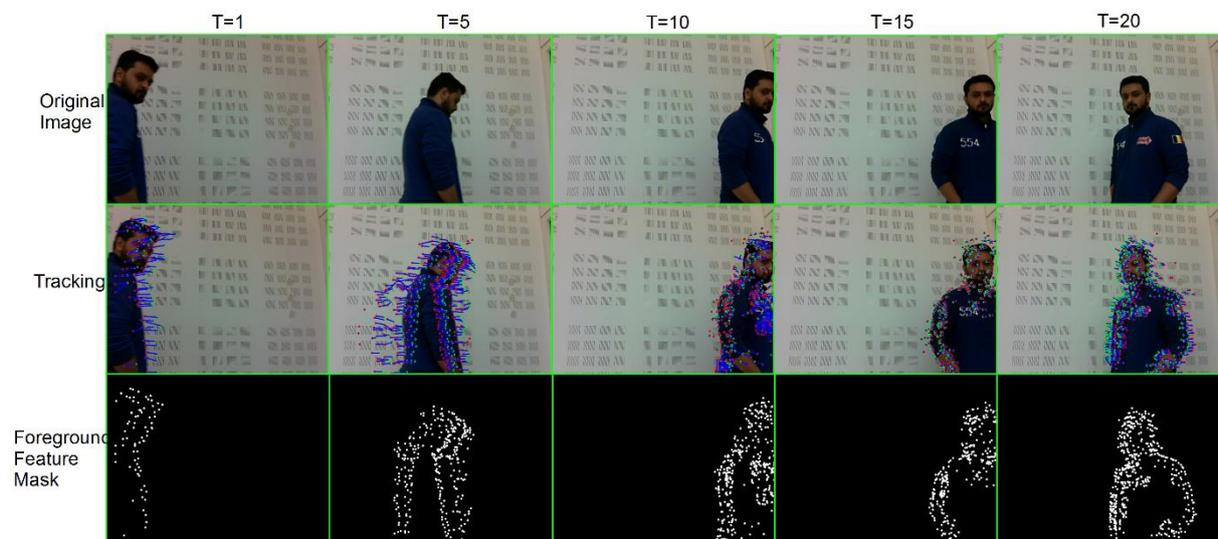
*Figure 5.5: Results from the proposed method of tracking motion input from the background subtraction module previously and clustering feature points. (Top row) original images, (middle row) tracking using Lucas-Kanade pyramid optical flow algorithm and (bottom row) foreground feature mask generated after tracking, clustering and segmentation*
