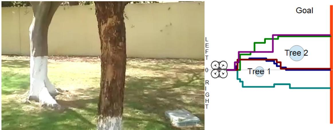
Figure 5.13: (Left) Frame consisting two trees as obstacles (Right) Drone flight path avoiding the trees in 5 successful runs using the proposed method
