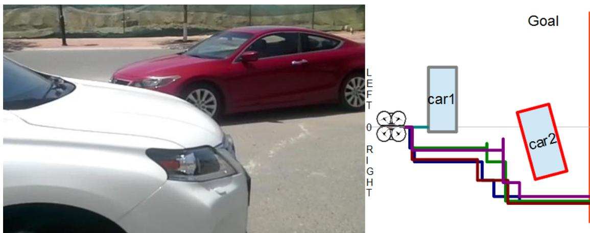
Figure 5.17: (Left) Frame consisting of two cars as wide obstacles. (Right) Drone flight path avoiding the trees in 4 successful runs and 1 failed run (turquoise) using the proposed method
