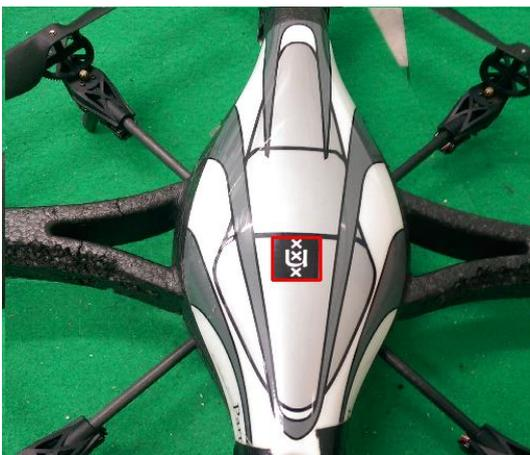
The red box over the result image is where the template matching method returns the best match in the source image. We use this method to compare current and previous images in our proposed method to estimate scale. We do this by generating several scaled versions of the template from the previous image and find the best match to the current image to determine the scale of expansion.
