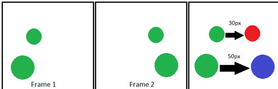
*Figure 3.6: Illustration of two balls rolling from left to right in Frames 1 and 2. The right frame shows the shift in pixels from Frame 1 to Frame 2 and segments them based on distance moved where the Blue ball is considered closer and the red ball considered further away from the camera.*
