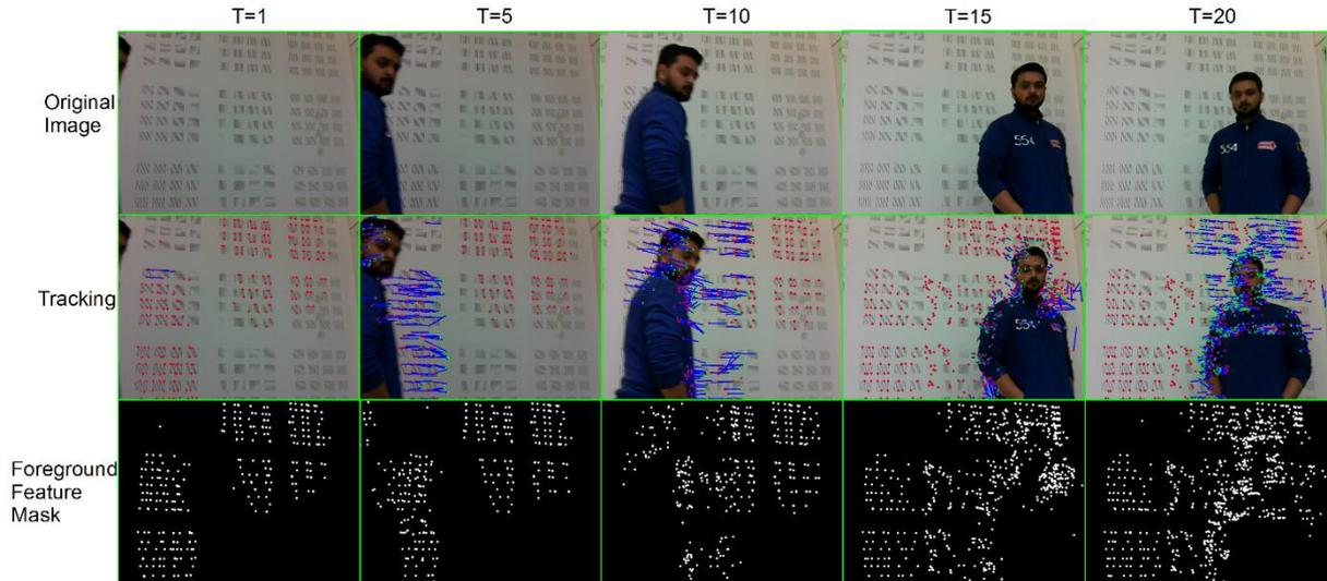
Figure 5.6: Results tracking step without using the proposed background subtraction step. (Top row) original images, (middle row) tracking using Lucas-Kanade pyramid optical flow algorithm and (bottom row) foreground feature mask generated after tracking, clustering and segmentation
