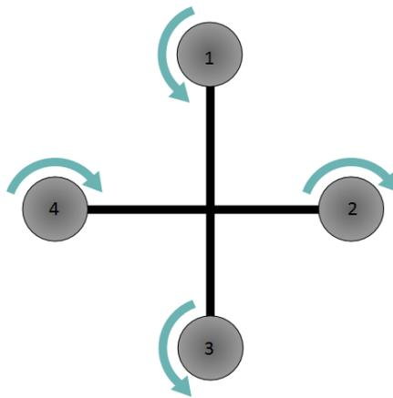
*Figure 5.2: Skeleton of a quad-rotor illustrating direction of rotation of each of the four rotors.*
