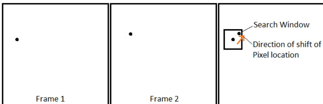
Figure 3.4: Illustration of Optical Flow of a moving pixel in consecutive images
