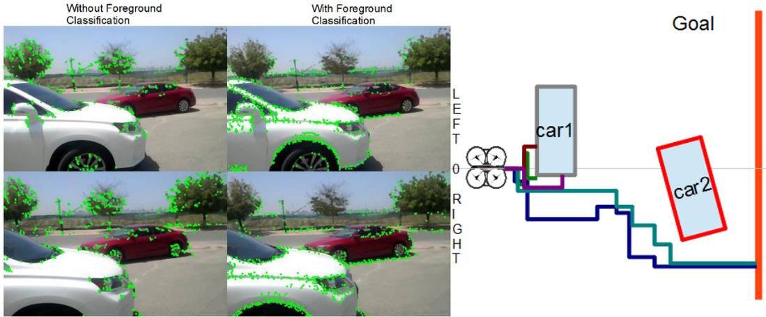
Figure 5.18: Drone flight frames illustrating results of the proposed method without Background/Foreground Classification (left) and with Background/Foreground Classification (middle) and flight results (right) avoiding 2 wide body obstacles
