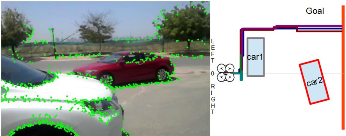
Figure 5.19: Drone flight results with 3 successful runs and 2 failed runs (green and turquoise) using only optical flow
