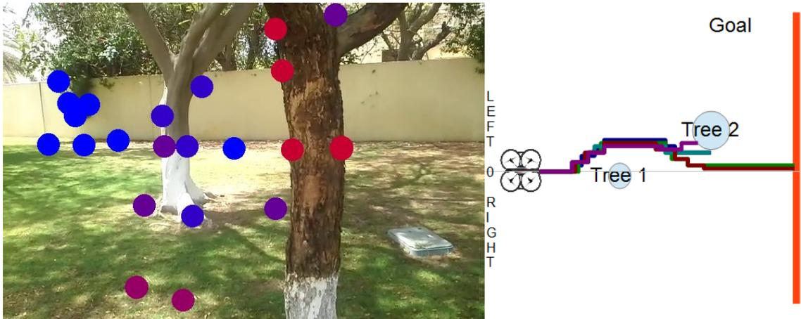
Figure 5.16: Drone Flight avoiding the trees in 2 successful runs using only proximity estimation
