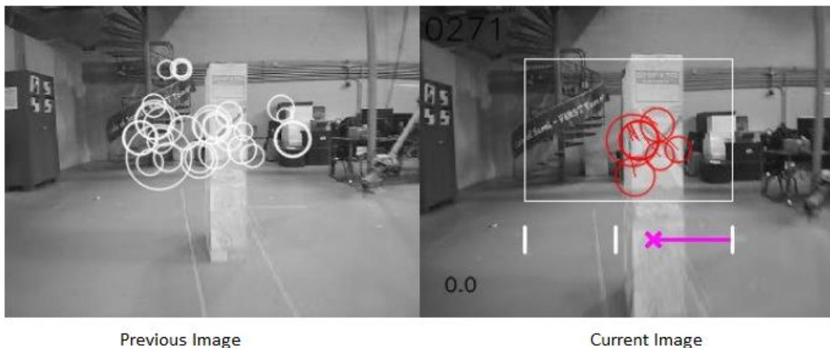
*Figure 2.1: Sample image of the expanding selected key points and command. The red circles represent the expanding key points. The purple line is the command given to the vehicle. One can see that many other key points in the field of view were rejected. Courtesy [24]*
