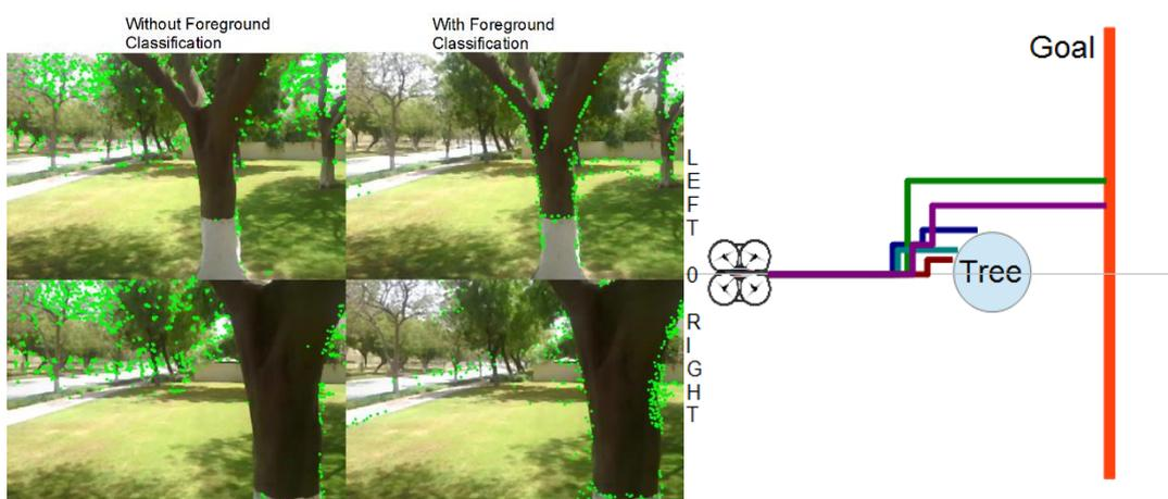
Figure 5.10: Drone flight frames illustrating results of the proposed method without Background/Foreground Classification (left) and with Background/Foreground Classification (middle) and flight results (right) avoiding 1 obstacle
