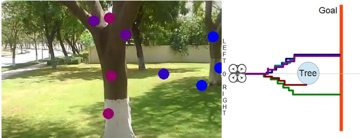
Figure 5.12: Drone Flight avoiding the tree in 4 successful runs using proximity estimation
