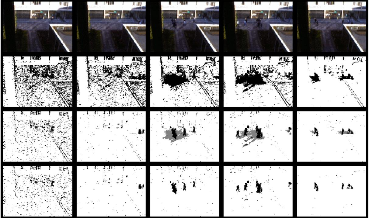
Figure 3.1: The top row consists of the original frame sequence at frames 15, 105, 235, 290 and 1200 respectively. The second row shows the results from Grimson *et al*'s. The last two rows are the result of the method proposed by Bowden *et al* where the white pixels are the background mask and the foreground is the black pixel regions without and with shadow removal. Courtesy [4].
