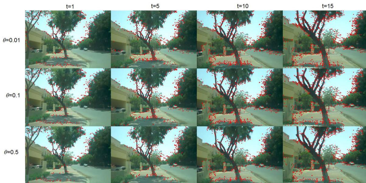
*Figure 4.5: Comparison of feature detection results at different corner score thresholds  $\theta$  for an outdoor scene*
