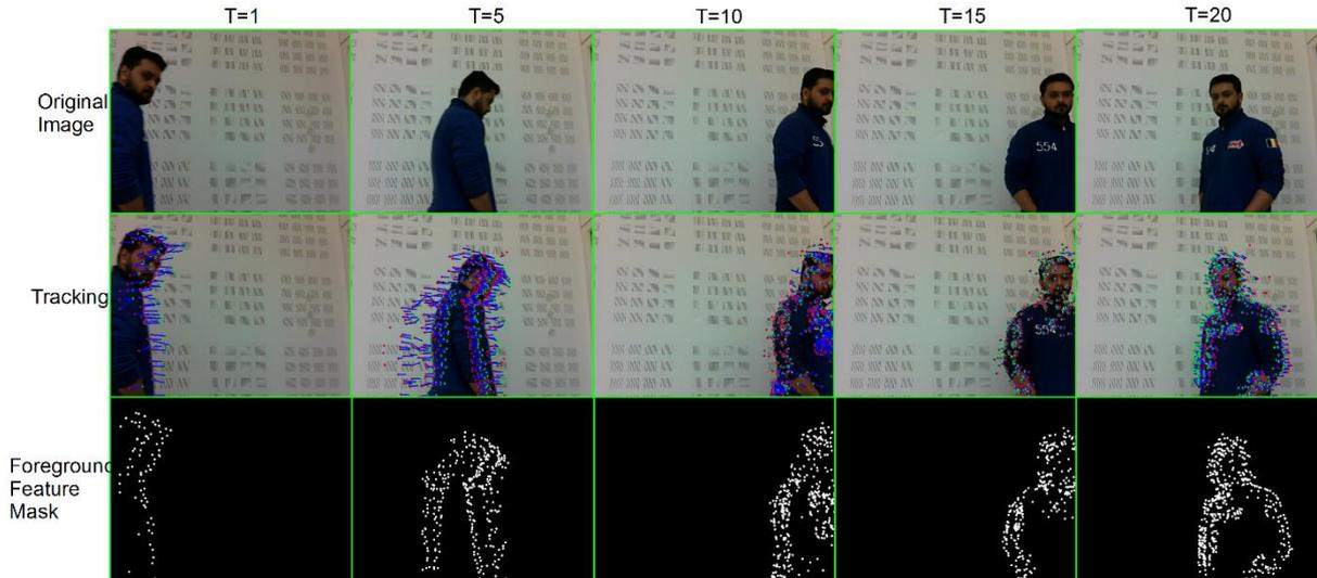
Figure 4.6: Results from the proposed method of tracking refined feature points. (Top Row) original images. (Middle Row) tracking using Lukas-Kanade pyramid optical flow method. (Bottom row) binary image showing location of feature points for clearer illustration.
