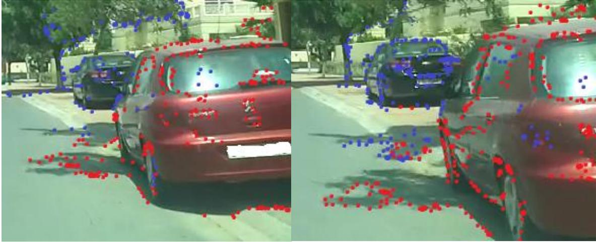
*Figure 4.8: Results of Depth estimation in a moving scene from Optical Flow. (Left) Frame at  $t=10$ . (Right) frame at  $t=14$ . Red dots denote features moving at a faster rate and Blue dots denote slower moving features*
