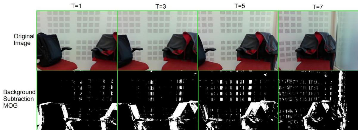
*Figure 4.2: Foreground mask generated from Background Subtraction using Mixture of Gaussians with the camera direction moving left to right in a fixed scene*
