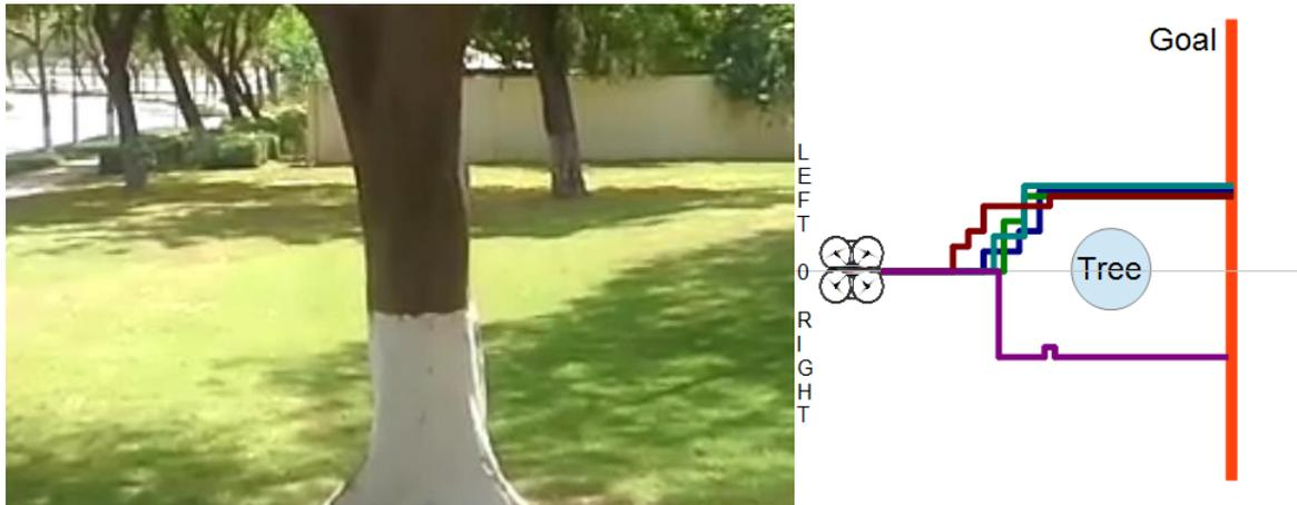
Figure 5.9: (Left) Frame consisting single tree as an obstacle. (Right) Drone flight path avoiding the tree in 5 successful runs using the proposed method
