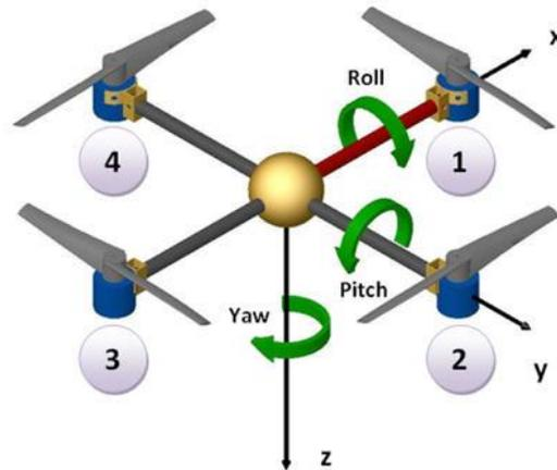
Figure 5.3: illustration of pitch, yaw and roll on quad-rotors
